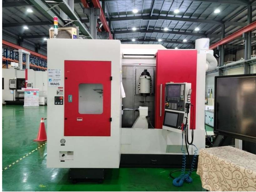
Figure 17: The target machine (Litz TM2500 5-axis turn mill machine)
